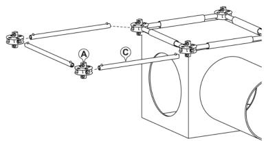
Ensure all holes in Joints (A) are oriented the same way as joints in Step 1.
