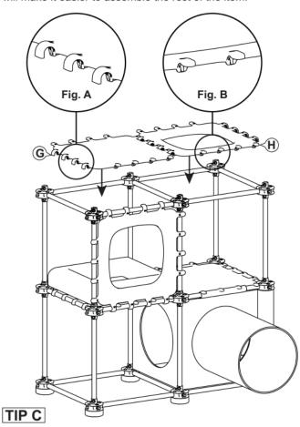
Ensure **Panels (G&H)** have clips and fingers oriented the same way as the panels in Step 6.
